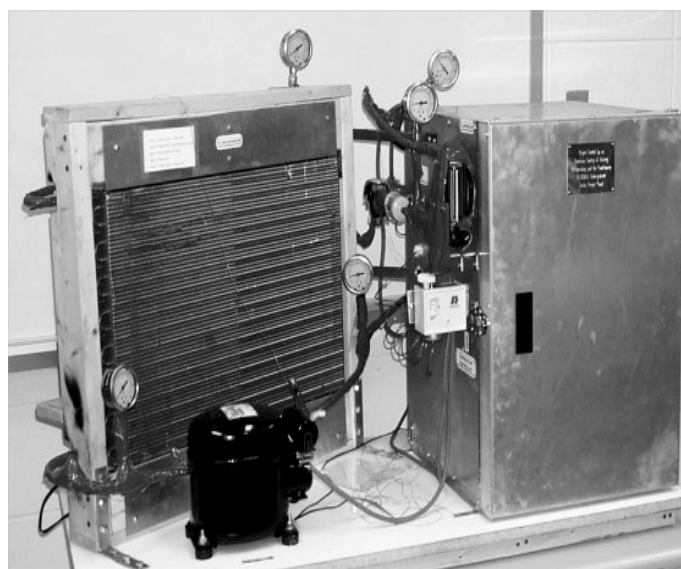
Figure 1: A Refrigeration System for a Small Compartment.
