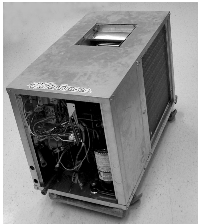
Figure 3: Heat pump water heater.
